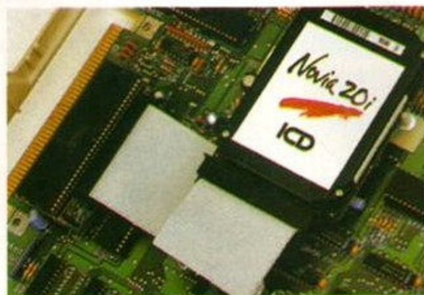
The Novia 20i is an internal hard drive for the Amiga 500: a useful, if very expensive, solution to A500 storage problems and unique... until now.
